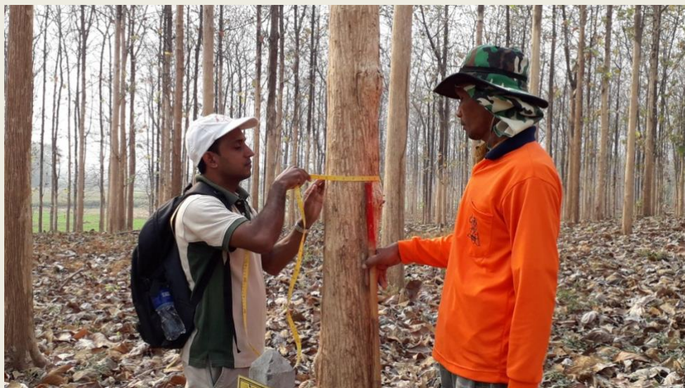
Figure 2.2: Diameter at breast height (1.3m) is measured by diameter tape. Inventory team follows all the standard and rules recommended in this regard.
